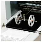
A powered exit conveyor ensures smooth ejection of folded paper.
