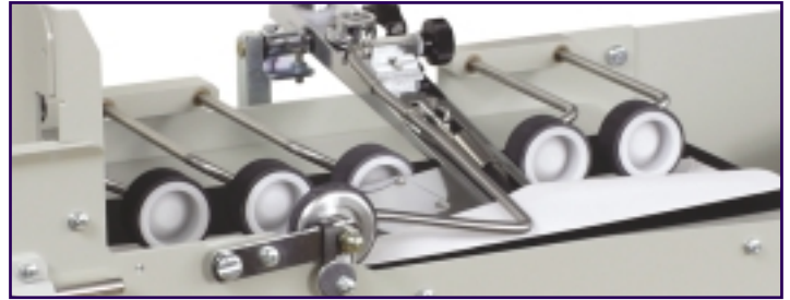
▲ Rubber conveyor belt has five transport rollers for a smooth take off and irreversible flow of envelopes
