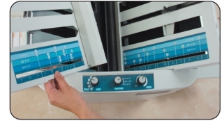
Split fold table permits removal
