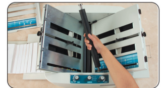
Removeable top roller
