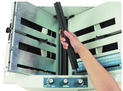
Removable top roller for easy maintenance
